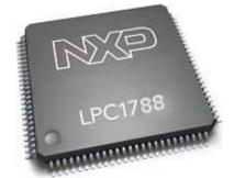
The NXP LPC1788 Cortex M-3 based microcontroller runs the open source uEZ<sup>®</sup> + FreeRTOS software platform. The LPC1788 has 512KB of internal Flash memory, 96KB of internal SRAM, a 10/100 Ethernet Media Access Controller (MAC), a USB full speed device/host/OTG controller, four UARTs, two CAN channels and a collection of serial communications interfaces. The uEZ GUI board also includes 8MB of external SDRAM and 8MB of external NOR Flash.
